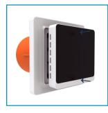
**4** Align the middle frame and the front cover with the installed back cover, then squeeze the top and bottom of the front cover back and forth with your fingers to make the front cover and the middle frame fit appropriately.
